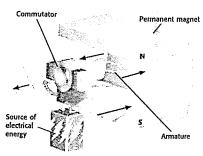
Running the Motor The commutator causes the electric current in the rotating armature to change directions. This causes the side that was pushed down to be pushed up and the other side to be pulled down. So the armature keeps rotating in the same direction.
