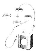
If no electric current is in the wire, the compass needles point in the same direction.
